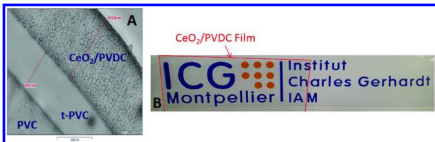
Figure 15. TEM picture of the section of a film prepared from a CeO 2 /PVDC hybrid latex (synthesized in the presence of poly(BA 4,8 -co-AA 4,9 ) RAFT oligomer) coated on a PVC support (A) and photography showing the transparency of the nanocomposite CeO 2 /PVDC film (B).
